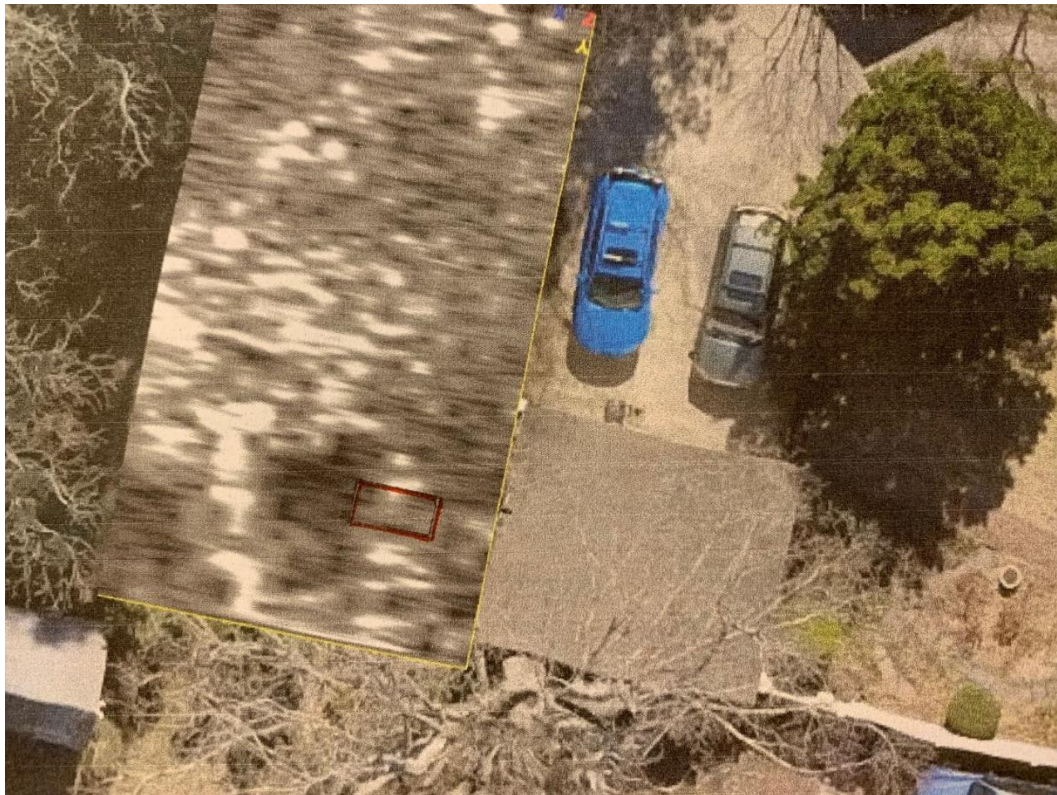
Aerial photo showing the GPR scan on the left at a depth of 1.5m with the trench location in red, and on the right the garage, with the cars waiting patiently outside.
